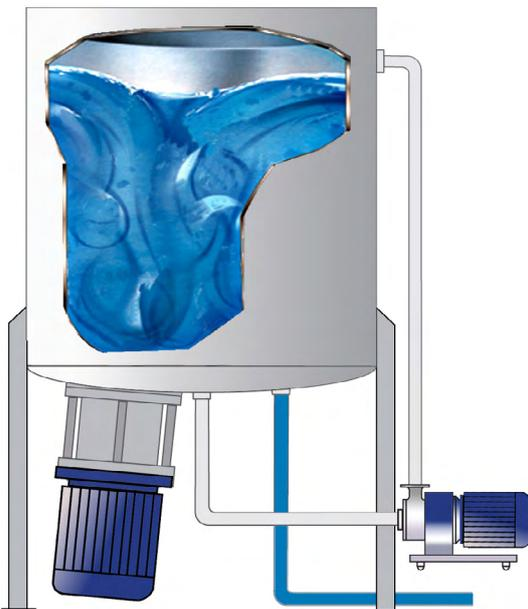
The intense high shear exerted on the polymer by the bottom entry and In-Line mixers ensures that particle size is minimised, exposing a greater surface area of polymer to the surrounding oil, allowing rapid solubilisation to be achieved. Samples can be drawn off to check dispersion and solubilisation is complete before the finished product is discharged.
